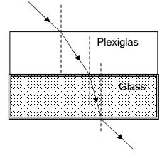
Faster in plexiglas – when light travels through glass the refracted ray bent further towards the normal meaning it is getting more slow in glass.
